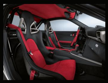
The interior also exudes the flair of sporting performance in virtually every detail, featuring lightweight bucket seats made of carbon-fibre-reinforced plastic in carbon surface finish and lightweight door panels with door opening straps. The basic interior colour is black, contrasting attractively with features such as the seat centre sections and the roof lining as well as segments on the steering wheel rim. The gearshift and handbrake lever are both finished in red alcantara.
